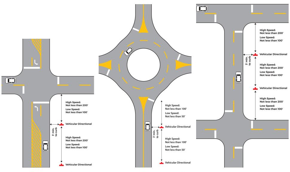
Intersection with Turning Lane Roundabout 4-Way & T Intersections
