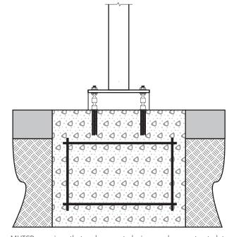
MUTCD requires that pole-mounted signage be constructed to breakaway standards. The illustration above shows a section of generic breakaway footer. Ultimately, final designs of footers, pole-mounting, and signs will be determined during the permitting and construction phase, based on the requirements of NC DOT and sign manufacturer's specifications.
